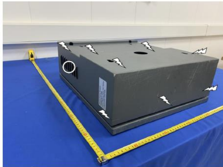
ESD discharge locations
